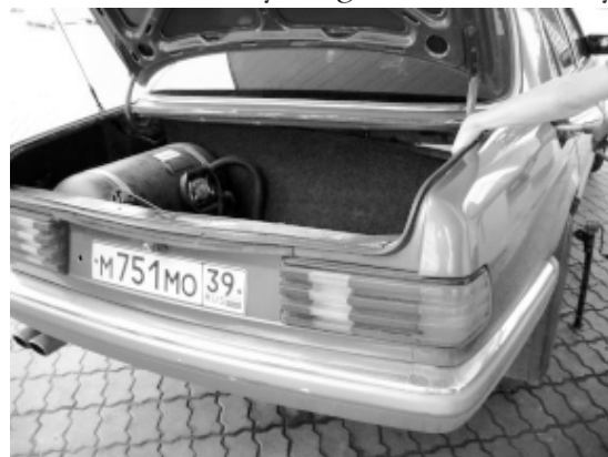
Gasoline is smuggled from the Kaliningrad Oblast to Poland in regular car tanks, while the car is powered from a liquid gas tank (photo: left side of the boot). In order to load a maximum of gasoline the car is lifted with a jack.
